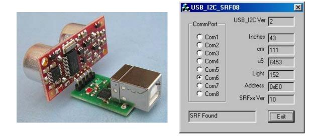
The connector on the USB-I2C module may be soldered directly to the SRF08 as shown, or you can use a cable if preferred. The USB-I2C module can easily supply the 25mA peak of the SRF08. The software
