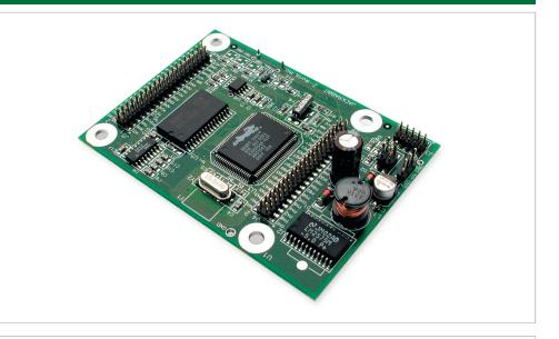
The BL1800 Jackrabbit is a small, easy-to-use, single-board computer that offers reliable hardware for embedded applications.
