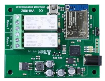
Factory reset jumper Bottom pair normal mode Top pair - Reset board
