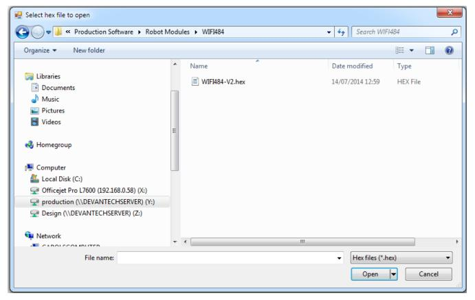
Once the file has been opened the programming sequence will now begin, it's fairly short and following it's completion the board will reset (automatically) and the LED will flash quickly while the programming sequence completes. Do not turn the power off in this sequence.
