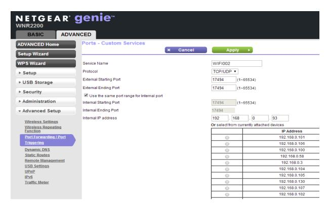
When applied you should now be able to talk to the router over the internet at the IP address designated by your internet provider. When a data packet arrives on port 17494 the router will pass the packet on to the local address on the network (192.168.0.93) on port 17494.
