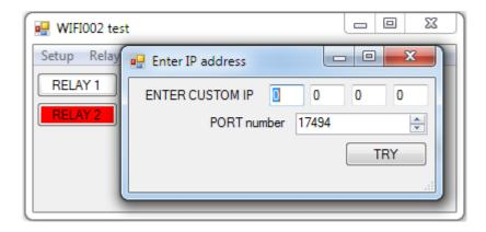
To test this you will need a computer that has its own internet connection and is NOT connected to the same network as the WIFI002. Download and run the <u>test program</u> above and select Custom IP. In the pop-up box enter your routers internet facing IP address. Click on "Try IP" and it will connect you to the WIFI002 just as if it were on your own network.
