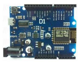
WeMos-D1R2 is an ESP8266-12 based WiFi enabled microprocessor unit on a Arduino-UNO footprint. That means the board looks and works (in most cases) like an UNO. Apparently several shields, sensors and output devices that are manufactured for the Arduino platform will work on the WeMos-D1R2 with the added advantage of built-in WiFi.
