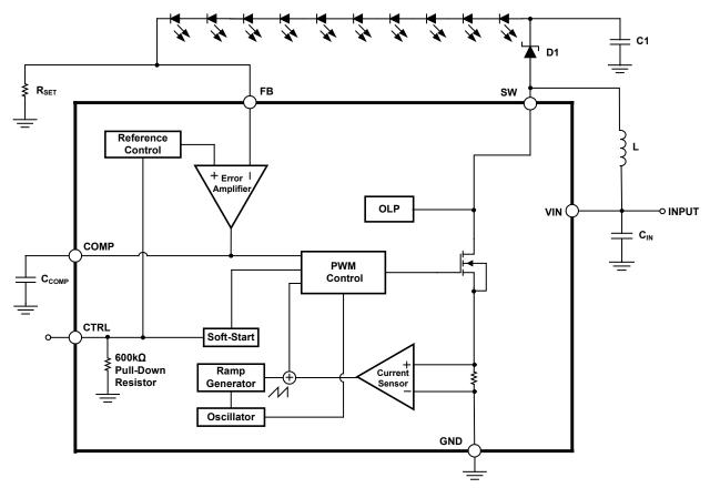
Figure 2. SGM3750 Block Diagram
