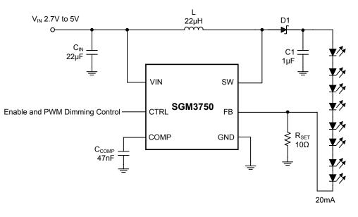
Figure 6. Li-Ion Driver for 8 White LEDs
