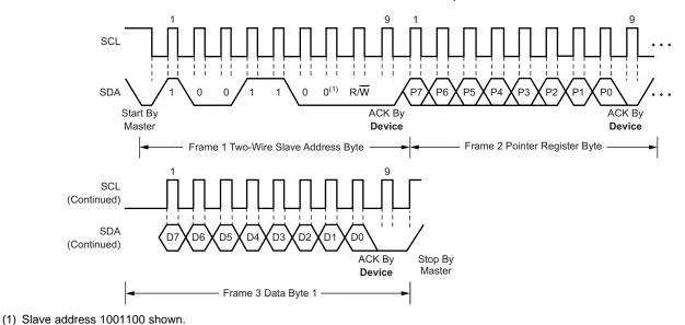
Figure 15. Two-Wire Timing Diagram for Write Word Format
