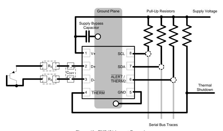
Figure 46. TMP451 Layout Example
