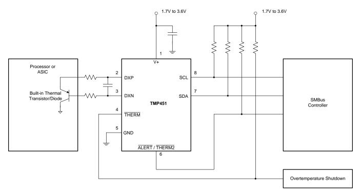
Figure 42. TMP451 Basic Connections Using a Processor Built-In Remote Transistor
