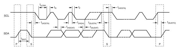
Figure 1. Two-Wire Timing Diagram
