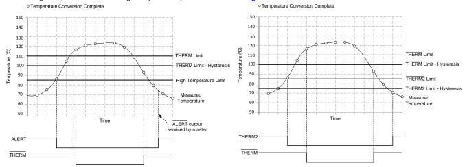
Figure 13. ALERT and THERM Interrupt Operation
