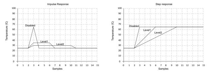
Figure 12. Filter Response to Impulse and Step Inputs
