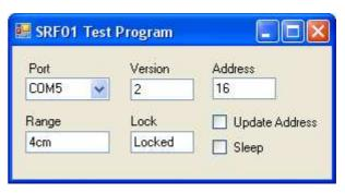
We have a small test program, written in C# which controls the SRF01 via the <u>Acroname S22</u> module. A small schottky diode is used to prevent the SRF01 trying to drive the S22's output line (data from the PC). You will need to download and install the <u>FTDI VCP</u> drivers to use the S22.
