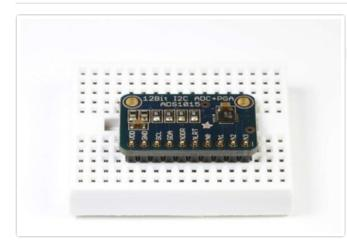
Position the breakout board Place the breakout board on the header pins.
