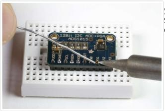
**Solder!** Solder each pin for a good electrical connection.
