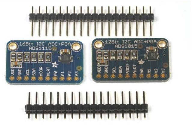
The ADS1115 and ADS1015 4-channel breakout boards are perfect for adding highresolution analog to digital conversion to any microprocessor-based project. These boards can run with power and logic signals between 2v to 5v, so they are compatible with all common 3.3v and 5v processors. As many of 4 of these boards can be controlled from the same 2-wire I2C bus, giving you up to 16 single-ended or 8 differential channels. A programmable gain amplifier provides up to x16 gain for small signals.
