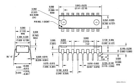
Molded Dual-In-Line Package (N) Order Number DM74ALS174N or DM74ALS175N NS Package Number N16A
