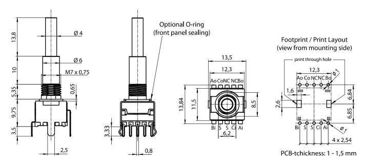
Both threaded and non-threaded bushings are available for all versions; THT vertical or THT horizontal (see type key).
