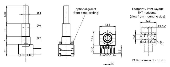
Both threaded and non-threaded bushings are available for all versions; THT vertical or THT horizontal (see type key).
