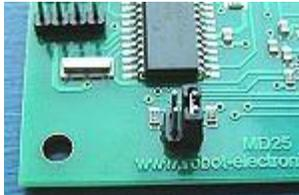
Serial mode at 9600 bps, 1 start bit, 2 stop bits, no parity
