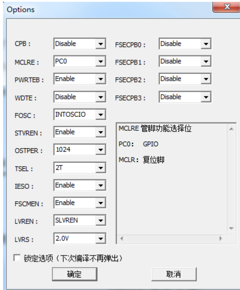
picture2-14 Chip Configuration Words (with FT61F14X example)
